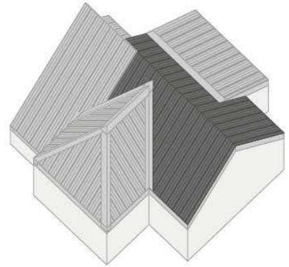
9. 5V Crimp Panels Install panels on high slopes (overlapping transition trim) and in any other un-paneled areas remaining.
