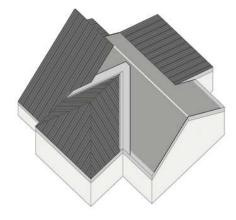
**5. Mighti-Rib Panels** Install panels, overlapping eave and valley trim. Do not fasten down panels along the ridge, if ridge trim is to be overlapped by the panels.
