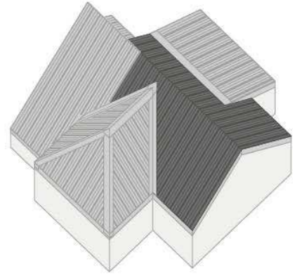
9. Standing Seam Panels Install panels on high slopes (overlapping transition trim) and in any other un-paneled areas remaining.
