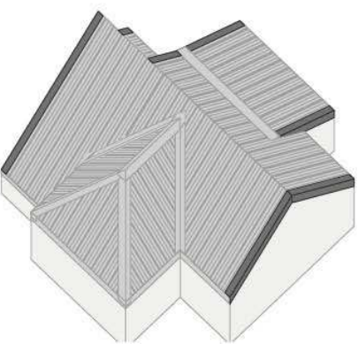
10. Gable/Rake Trim Install gable trim (rake trim) along all gable (rake) edges, overlapping panels.
